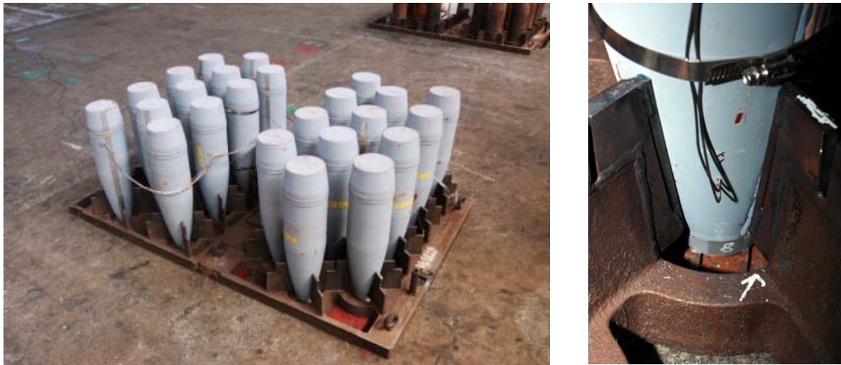
Figure 3 – TRRP Mmunition Test Tray with Coldest Munition Thermocouple Installed
